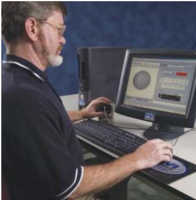
FIGURE 2. FiberQA-EFI is a semi-automated system that allows manufacturers of fiberoptic connectors to accurately detect and classify end-face defects such as scratches, pits, particles, blemishes, and chips. This system semi-automates the process of identification and measurement of fiber geometries, which improves quality control in the manufacturing process.
